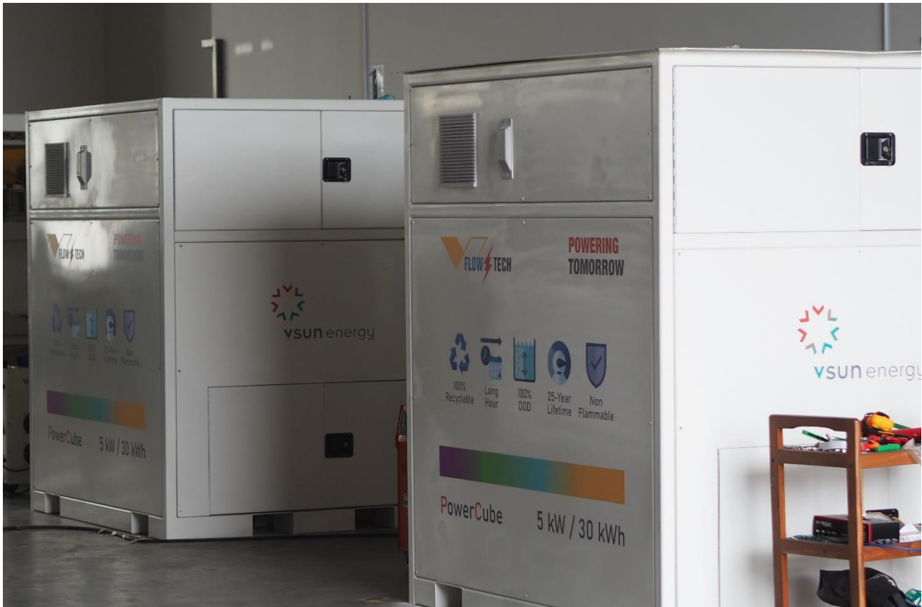
Figure 1 VSUN Energy branded V-Flow Tech 5kW/30kWh VRFBs
