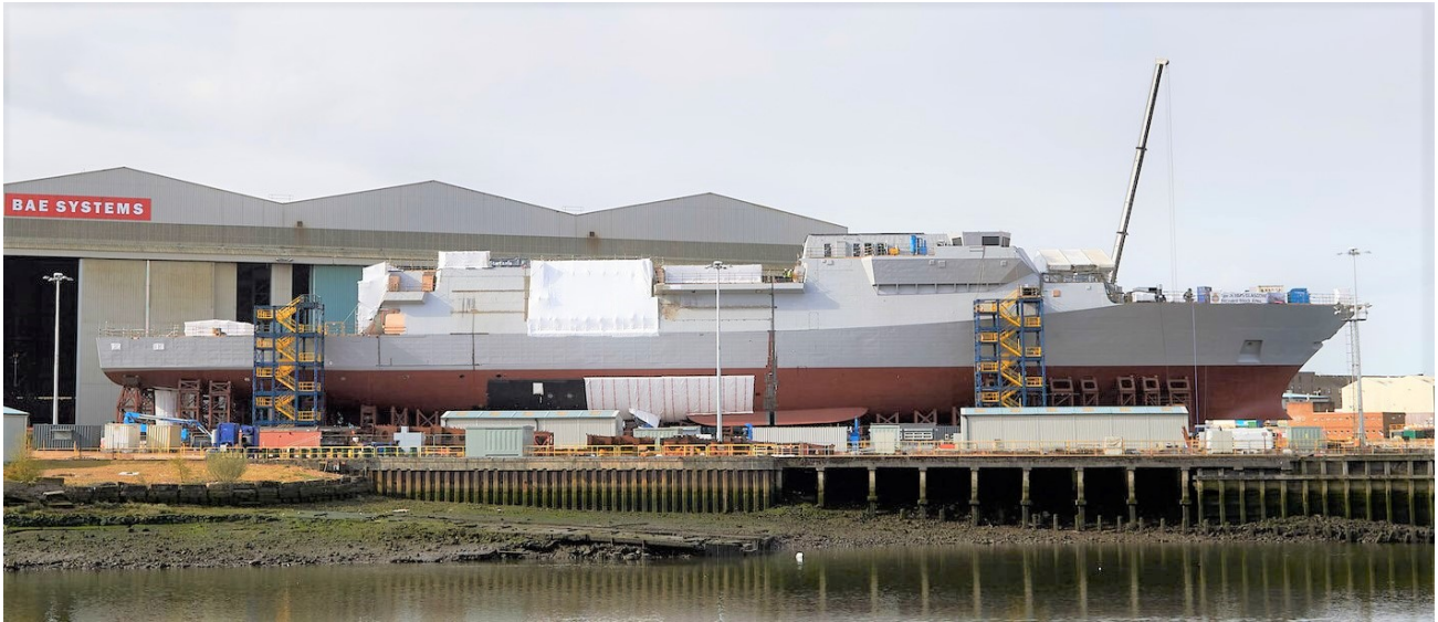
A BAE Systems Type 26 Frigate, HMS Glasgow, under construction. The Type 26 Frigate is the reference ship design for the Hunter Class Frigates.
