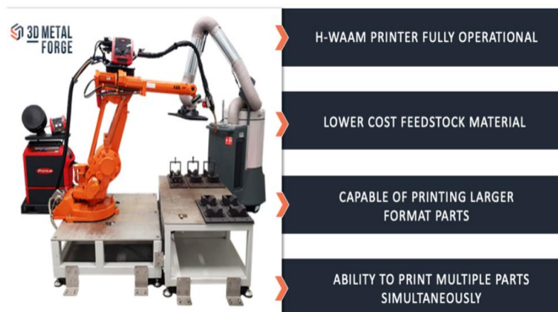
Image of Hybrid Wire Arc (H-WAAM) printer at PSA facility
