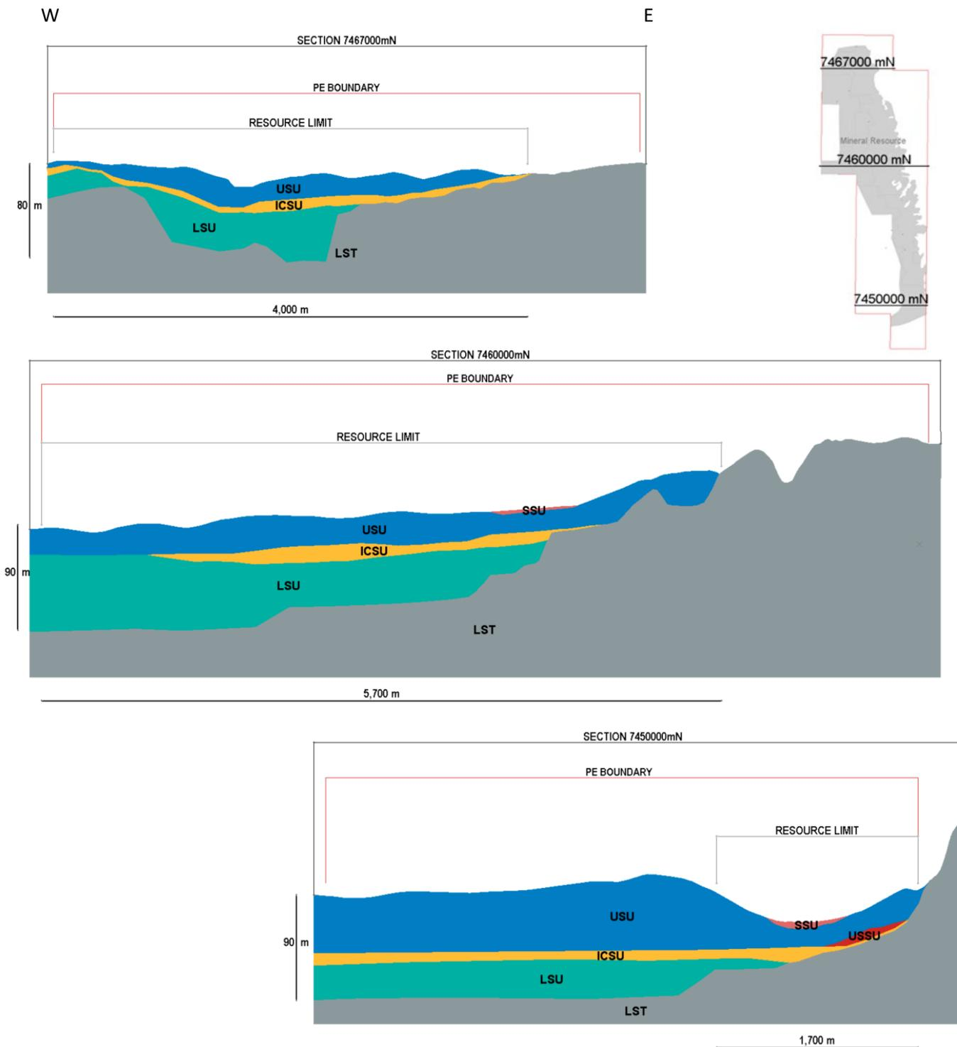
Notes: Sections plotted with 10 x vertical exaggeration looking North (L is West, R is East), PE Boundary = Mining Lease, geology interpretation from drill logs
