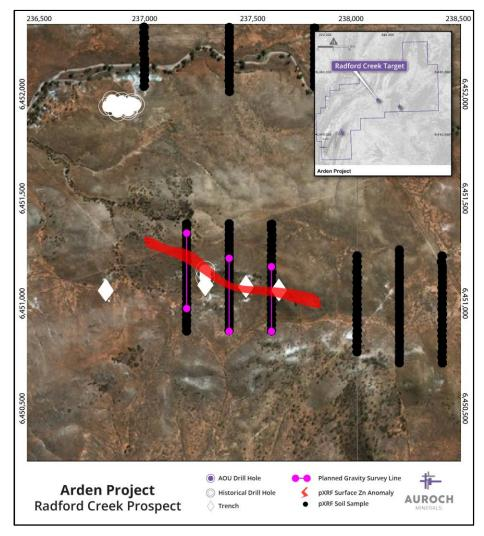
Figure 2 – Planned gravity survey lines over the surface zinc anomalies at the Radford Creek prospect at Arden.
