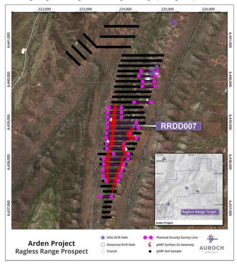
Figure 1 – Planned gravity survey lines over the surface zinc anomalies at the Ragless Range prospect at Arden.
